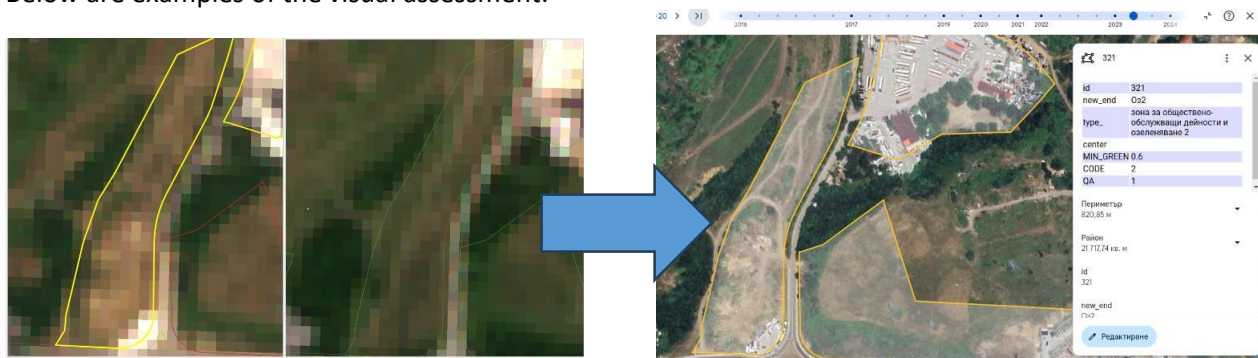
Fig. 2. Quality assessment. Left: Visual analysis of Sentinel-2 images between 2017 and 2023 with observed visible change in the condition of green areas. Right: Confirmation of the observed change using very high-resolution archival images in Google Earth Engine.
